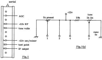
A favourite tuner used extensively by amateurs is the Mullard ELC1043 and ELC1043/05. These are readily available and inexpensive, the later versions may not quite tune down as low as the 70cm band but by a simple modification can be made to do so. The tuners as purchased are quite sensitive and suitable for receiving
