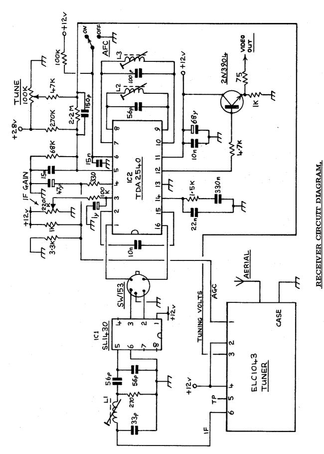
The tuner can be a modified ELCIO43 commercial type, the broadband converter shown elsewhere in this chapter or any other tuner having an IF frequency of 39.5 MHz. The tuner IF output is matched to the IF preamplifier (IC1) with the tuned circuit L1/C1, R1 ensures correct broadband termination.
